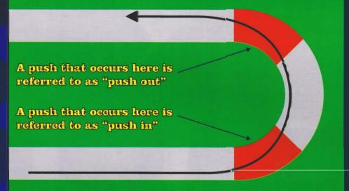
Immediately can see that one of the four describes a problem getting into the corner (push in), one of the remaining three describe a condition where the kart won't turn (push out), and the final two describe conditions where the kart will turn but it's not fast (kart on the LR or RR). These same final two also describe two conditions which are caused by the exact opposite
